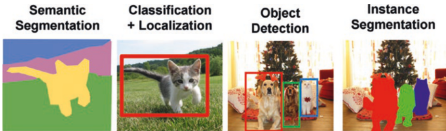
Figure 6-1. A visual explanation of the different terms describing the general task of locating one or more objects in an image
