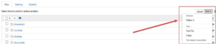
Figure 1-9. To create a new notebook, click on the New button located on the top-right part of the page and choose Python 3
