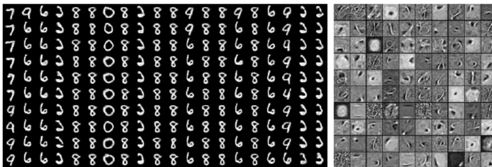
Figure 16.15: Samples from a trained RBM, and its weights. Image reproduced with permission from LISA (2008) . (Left) Samples from a model trained on MNIST, drawn using Gibbs sampling. Each column is a separate Gibbs sampling process. Each row represents the output of another 1,000 steps of Gibbs sampling. Successive samples are highly correlated with one another. (Right) The corresponding weight vectors. Compare this to the samples and weights of a linear factor model, shown in figure 13.2. The samples here are much better because the RBM prior p(\mathbf{h}) is not constrained to be factorial. The RBM can learn which features should appear together when sampling. On the other hand, the RBM posterior p(\mathbf{h} | \mathbf{v}) is factorial, while the sparse coding posterior p(\mathbf{h} | \mathbf{v}) is not, so the sparse coding model may be better for feature extraction. Other models are able to have both a non-factorial p(\mathbf{h}) and a non-factorial p(\mathbf{h} | \mathbf{v}) .
