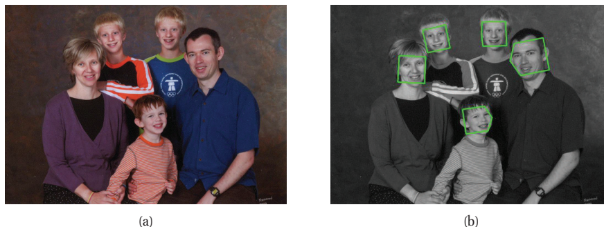
Figure 1.6 Example of face detection. (a) Input image (Murphy family, photo taken 5 August 2010). Used with kind permission of Bernard Diedrich of Sherwood Studios. (b) Output of classifier, which detected 5 faces at different poses. This was produced using the online demo at http://demo.pittpatt.com/ . The classifier was trained on 1000s of manually labeled images of faces and non-faces, and then was applied to a dense set of overlapping patches in the test image. Only the patches whose probability of containing a face was sufficiently high were returned. Used with kind permission of Pittpatt.com
