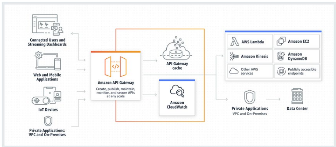
Figure 1-10. Architecture of API Gateway
