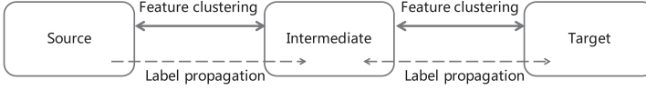
Figure 11.5 An illustration of the CMTF algorithm in the TTL framework. The algorithm learns two coupled feature representations by feature clustering, and then propagates the label information from the source domain to the target domain through the intermediate domain based on the coupled feature representation
