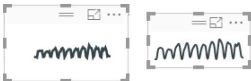
Figure 7-34: A couple of examples of the same chart, using a standard line chart and a sparkline custom visualization.
