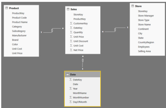
Figure 6-3: The data model structure is a very simple schema, with Sales in the middle and the other tables around it.
