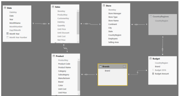
Figure 6-15: Among the many relationships, the one between Brands and Budget is inactive, signified by the dashed connector line between them.
