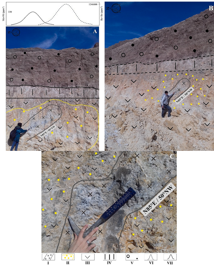
Fig. 9. Exploration of Buried and hidden mineralization in the eastern part of zone G2 in the Gandy deposit. I- Mineralization (orebody), II- Primary halo, III- Bedrock, IV- Weathering crust (Soil) and secondary residual halo, V- Alluvium, VI- The multiplicative indicator of supra-ore elements (Ba × Ba), VII- The multiplicative indicator of sub-ore elements (Mo × Ni).
