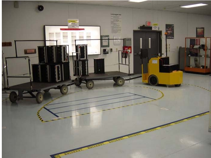
Tow motor route controlled through floor markings.
