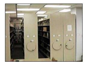
Sensors are placed on the floor between the shelves & will not allow the shelves to be closed when activated
