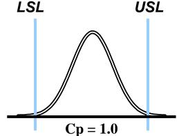
□ A Cp of 1 indicates that the width of the process and the width of the specification are the same.
