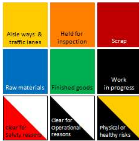
Standard Floor Markings
