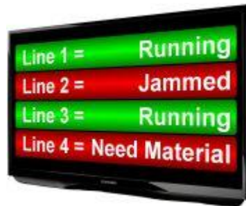
Fig. 3. a) workstation signaling element in andon system, b) andon board
