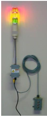
Fig. 3. a) workstation signaling element in andon system, b) andon board
