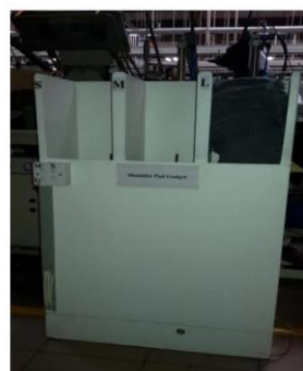
Figure16: Isometric View of Shoulder Pad Gadget & Keeping Shoulder Pads in the Gadget
