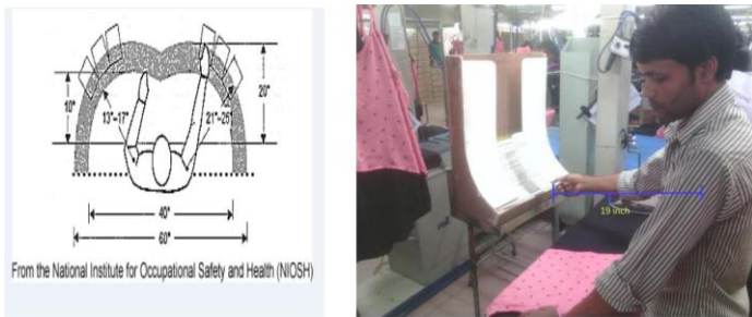
Figure 18: Comfortable Zone for Work Proposed by NIOSH in Respect to Hanger Box
