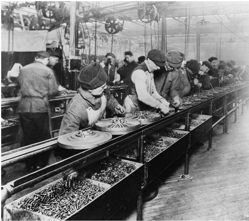
FIGURE 13.8 Ford magneto assembly line in Highland Park, 1913.
