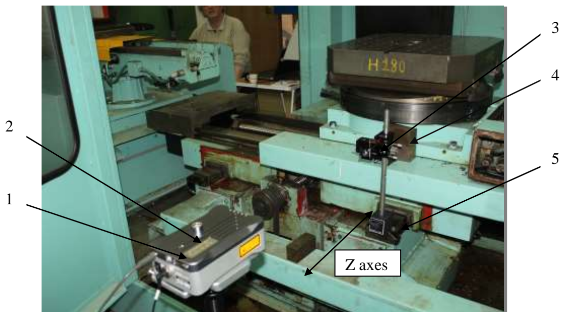
Figure 2.2.8. The linear measurement on Z Axis at the Flexible Manufacturing Cells UO-01 FMC realized by XL 80 laser [20]
