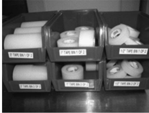
FIGURE 6.19 Two-bin Kanban system example: Operators take from top bin first. An empty bin signals replenishment needed. Drawback to this setup is operators can draw from both bins and could have FIFO issues when second bin is returned. Source: BIG Archives.
