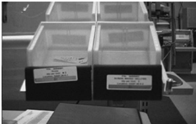
FIGURE 6.20 Two-bin system operator draws from first bin then 2nd bin slides down. The first bin is the signal to replenish. Operators could still draw from second bin but this bin setup is more clear. Source: BIG Archives.
