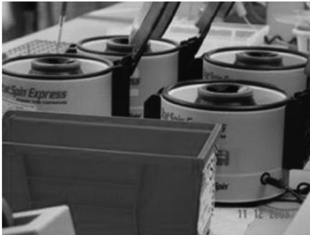
FIGURE 2.2 Lab Mini Centrifuges located at the machine point of use (POU). Source: BIG Archives.
