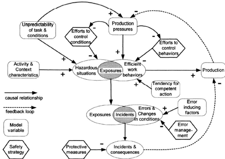
Figure II.10 - Systems Model of Construction Accident Causation (Mitropoulos et al. 2005)
