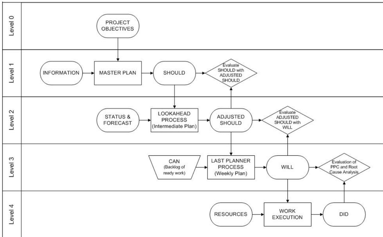
**Figure II.5 - The Last Planner System (adapted from Howell and Ballard 1994)**
